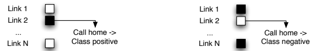
(a) Detecting links in an OR class. The server is signalled by the first visited link. Note that subsequent visited links will not signal the server, as they will be handled by browser cache; thus, the server cannot tell how many of the links were visited.
